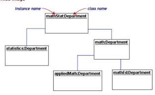
Each rectangle in the object diagram corresponds to a single instance. Instance names are underlined in UML diagrams. Class or instance names may be omitted from object diagrams as long as the diagram meaning is still clear.
