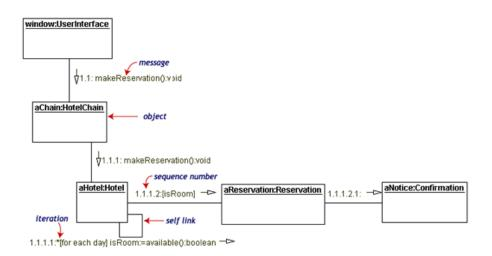
The object-role rectangles are labeled with either class or object names (or both). Class names are preceded by colons (:).
